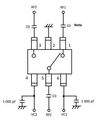
Note C0 : 0.05 to 0.5 GHz 1,000pF : 0.4 to 2.0 GHz 56pF : 2.0 to 3.8 GHz 8pF
